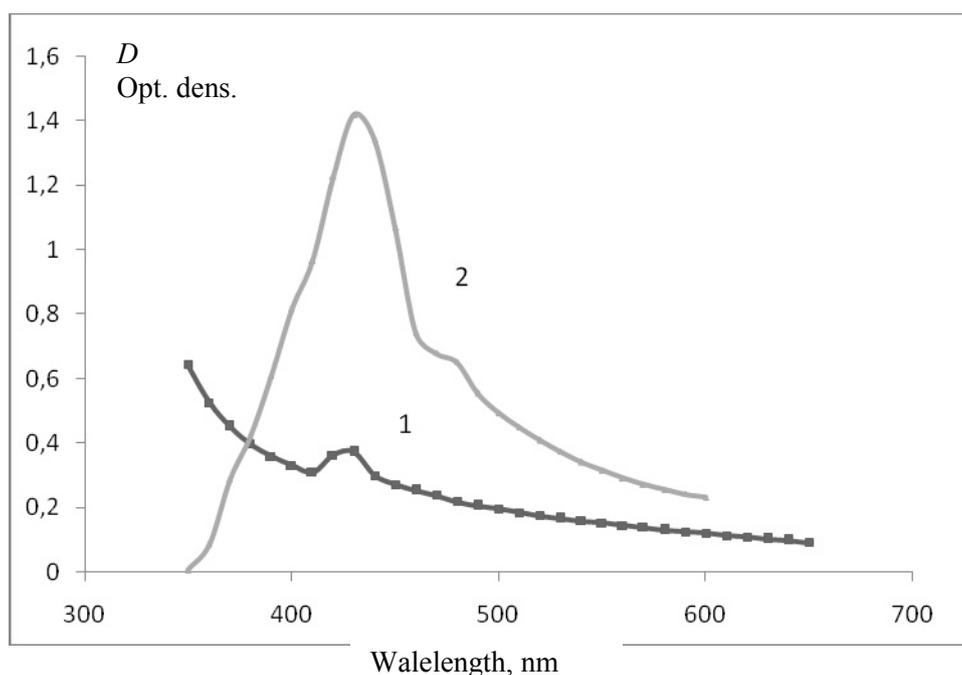
Figure 6. Absorption spectrum of nanoparticles of silver: after repeated dissolution (1), in initial solution before introduction of particles of silver (2)
