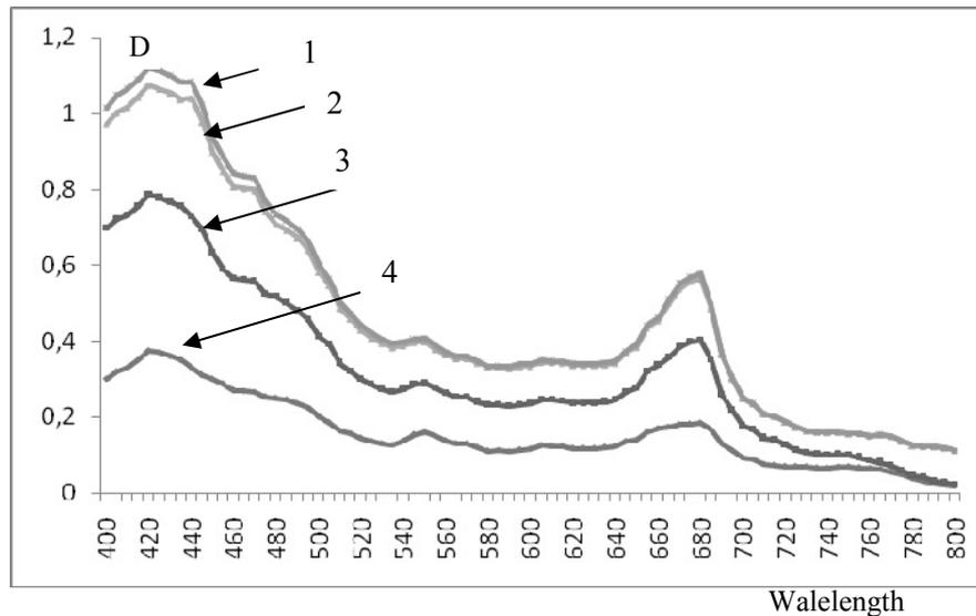
Figure 5. Absorption spectra of solutions of a green leaf at different concentration of chlorophyll. Increase of concentration of chlorophyll comes from a curve 3 to a curve 1
