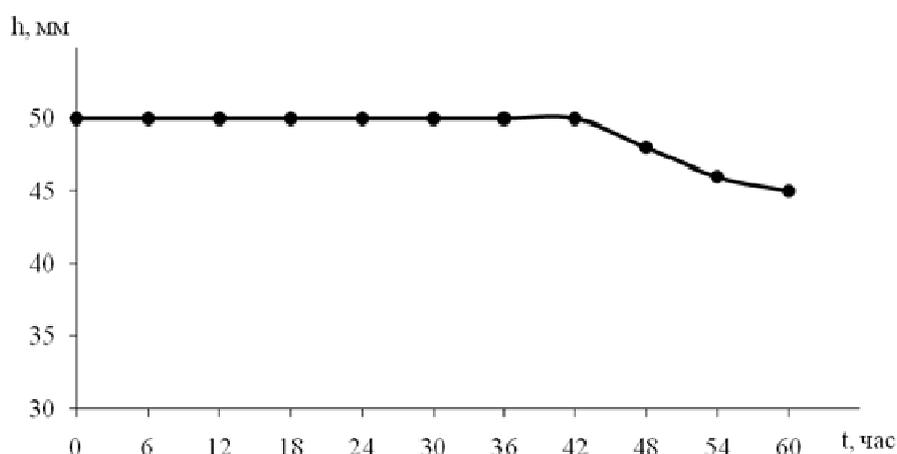
Figure 6. Dependence of the height of the dispersed phase layer on the time of the suspension with the addition of sodium humate
