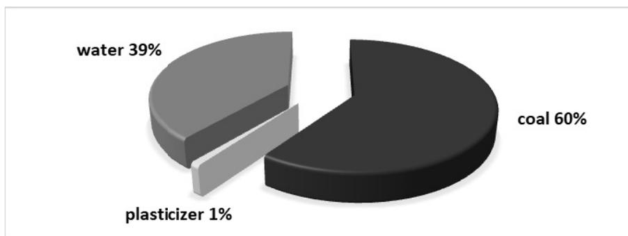
Figure 2. Percentage in a coal-water suspension with a mass fraction of the solid and liquid phase
