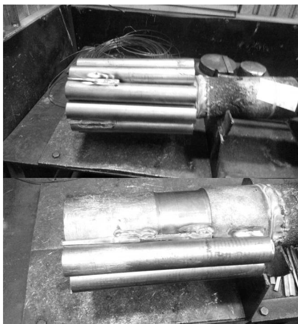
Figure 1. A photograph of the consumable electrode for FGWP
