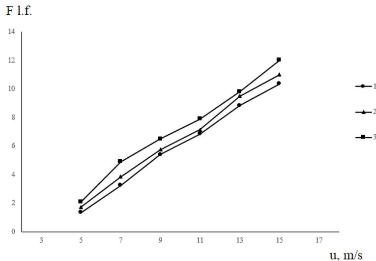
Figure 4. Graph of the dependence of the drag force of a rotating cylinder on the change in the air flow velocity and on  $k/d$ : 1) 0.005, 2) 0.01, 3) 0.02
