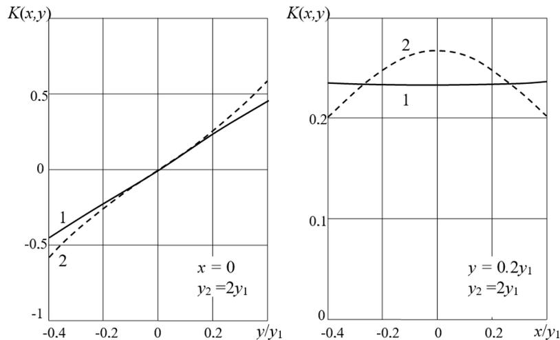
Figure 8. Dependence of the coordinate factor  $K(x,y)$  on the change in the measured coordinate of the conductor axis  $y(a)$  and on the change in the orthogonal coordinate  $x(b)$  for the proposed transducer (1) and the prototype transducer (2)
