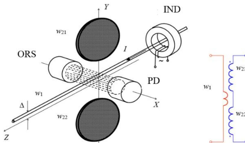
Figure 6. Design of the inductive-optical transducer: *ORS* — optical radiation source; *PD* — photodetector; *IND* — inductor;  $w_1$  — conductor with current (excitation winding);  $w_{21}$ ,  $w_{22}$  — measuring winding sections
