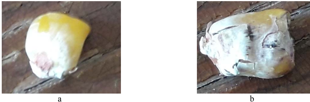
Figure 5. Appearance of maize seed at a vacuum of 60 kPa (a) and a vacuum of 45 kPa (b)
