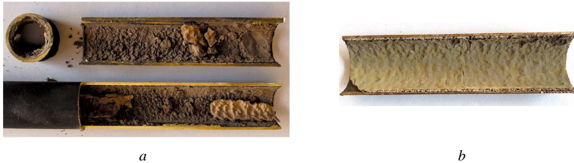
Figure 2. Samples of heat exchange pipes sections from CHPP-3 after operation during the heating season: a) — boiler pipe, d=19\text{mm} ; b) — condenser pipe, d=28\text{mm}
