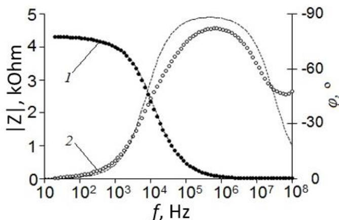
Figure 2. Frequency dependences of impedance modulus  $|Z|$  (1) (●) and  $\varphi$  phase angle (2) (○) for serial ceramic samples of composition BeO + 30 wt. %,  $T = 1530$  °C
