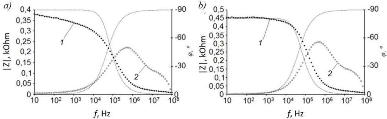
Figure 3. Typical frequency dependences of impedance modulus  $|Z|(1)$  ( $\bullet$ ) and  $\varphi$  phase angle (2) ( $\circ$ ),  $T = 1550\text{ }^\circ\text{C}$ : a) (P.2)  $\text{BeO} + 29,5\% \text{TiO}_2^{\text{um}} + 0,5\% \text{TiO}_2^{\text{nano}}$ ; b) (P.4)  $\text{BeO} + 28,5\% \text{TiO}_2^{\text{um}} + 1,5\% \text{TiO}_2^{\text{nano}}$ .
