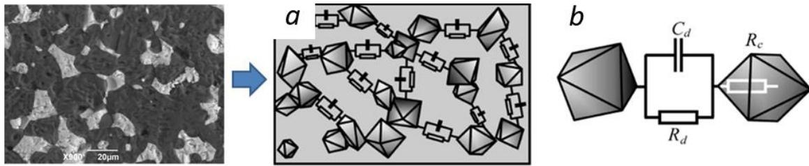
Figure 8. Schematic representation of the composite material structure [21] (in the inset on the left is an electronic image of the microstructure of a ceramic sample of composition P.3): a) up to the flow threshold; b) equivalent substitution scheme
