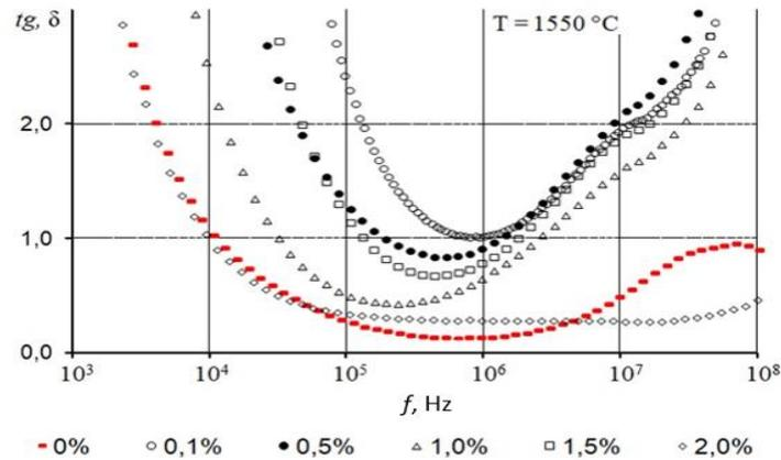
Figure 7. Frequency dependence of the dissipation factor on the content of TiO<sub>2</sub> nanoparticles, T = 1550 °C (P.1 — P.5)
