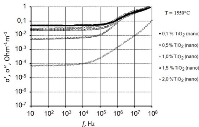
Figure 5. Frequency dependence of actual  $\sigma'$  component of specific conductivity as a function of  $\text{TiO}_2$  nanoparticles content,  $T = 1550\text{ }^\circ\text{C}$  (P.1 — P.5)
