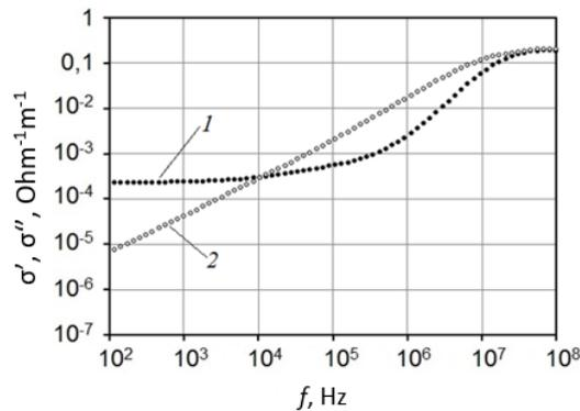
Figure 4. Frequency dependence of actual  $\sigma'$  (1) and imaginary  $\sigma''$  (2) components of specific conductivity of serial ceramics (P.0) of  $\text{BeO} + 30\% \text{TiO}_2^{\text{um}}$ ,  $T = 1530\text{ }^\circ\text{C}$
