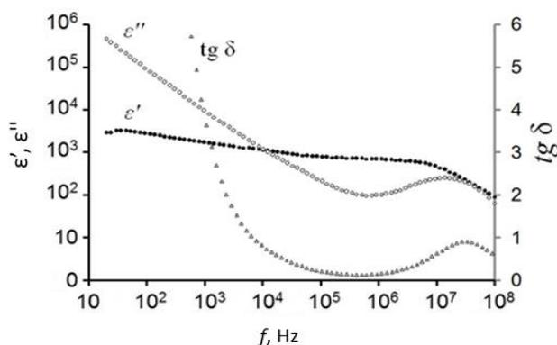
Figure 6. Variation curves of values of the actual and imaginary components of dielectric permittivity, dissipation factor for the factory sample composition:  $\text{BeO} + 30\% \text{TiO}_2^{\text{nm}}$ ,  $T = 1530\text{ }^\circ\text{C}$  (P.0)
