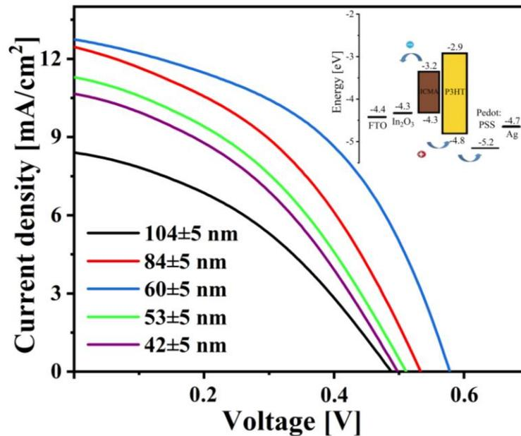
Figure 5. Current-voltage characteristic of a polymer solar cells In<sub>2</sub>O<sub>3</sub>/P3HT: ICMA/ PEDOT: PSS/Ag
