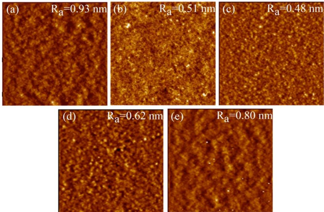
a) 1500 rpm; b) 2000 rpm; c) 3000 rpm; d) 4000 rpm; e) 5000 rpm.
