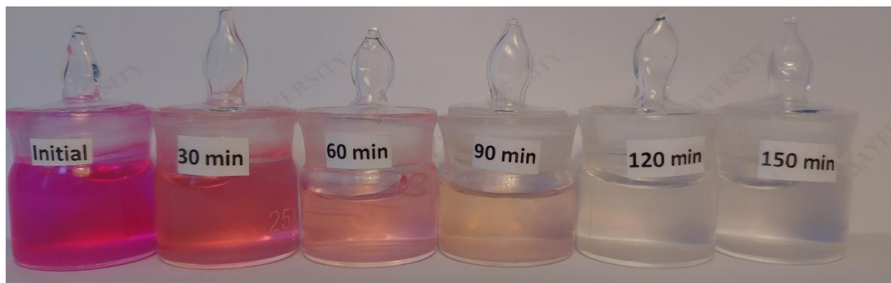
Figure 5. Photo of RhB solution in the presence of # 3 after each 30 min of UV exposure
