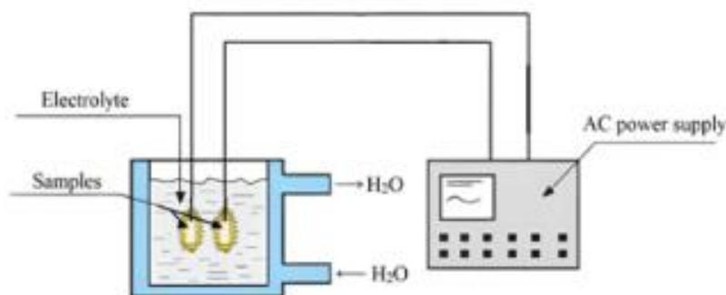
Figure 1. Schematic diagram of the MAO device
