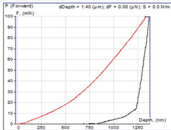
Figure 7. Dependence of indenter penetration depth on applied force in calcium-phosphate-coated titanium VT1-0 sample when 1 g titanium oxide is added to the electrolyte
