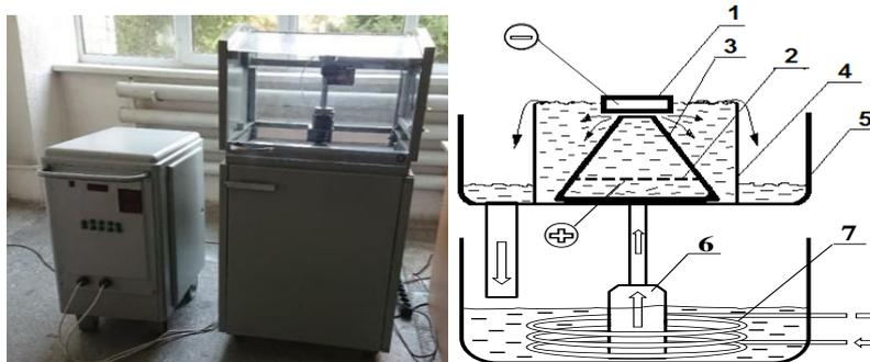
1 — sample to be treated (cathode), 2 — stainless steel anode with holes, 3 — cone-shaped partition, 4 — working chamber — bath with electrolyte, 5 — pan, 6 — pump, 7 — heat exchanger
