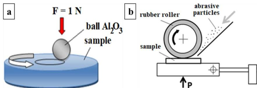
a — according to the scheme “ball on disk”, b — according to the scheme “rotating roller — plane surface”
