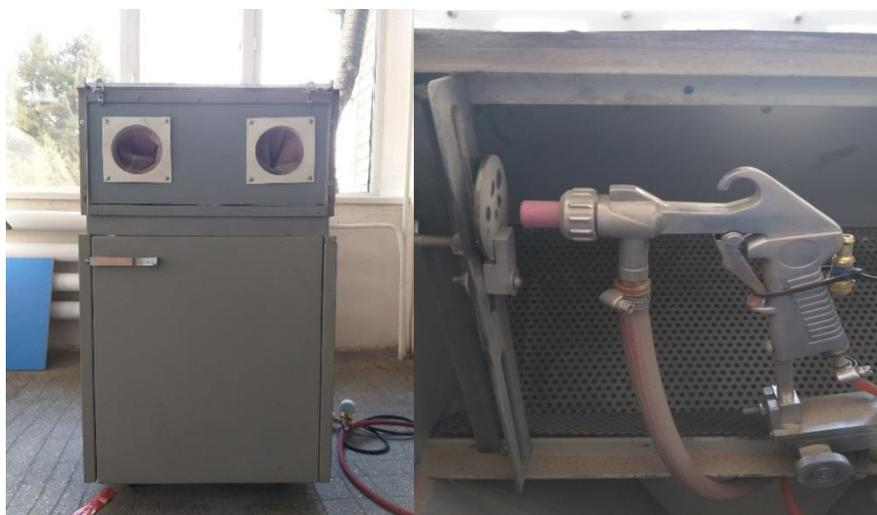
Figure 4. Bench for erosion testing
