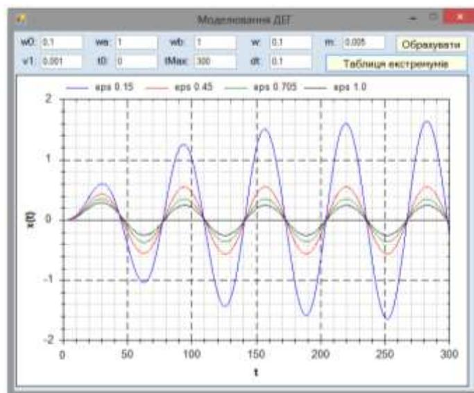
Figure 4. Interface of the computer program for simulating the operation of two-channel TG under the action of external perturbing accelerations
