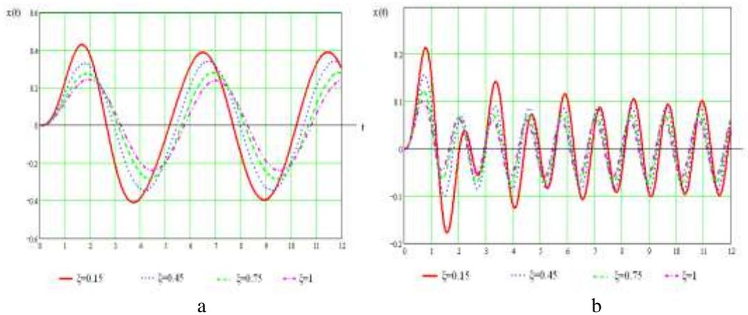
Figure 7. Two-channel TG output plot for different damping ratios  $\zeta$  at  $w_a = w_b = 3 \text{ m/s}^2$  and  $\omega = \omega_0/5 = 0,05 \text{ s}^{-1}$  (a) and  $\zeta$  at  $w_a = w_b = 3 \text{ m/s}^2$  and  $\omega = 2\omega_0 = 0,2 \text{ s}^{-1}$
