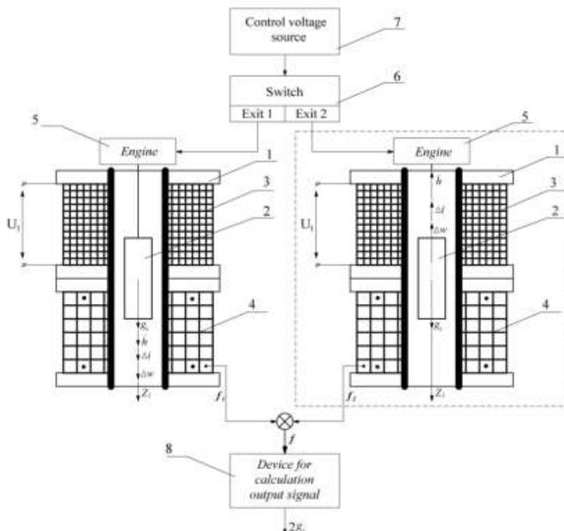
Figure 3. Block diagram of the new two-channel TG [7]
