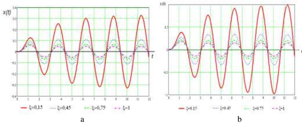
Figure 6. Plot of two-channel TG output signal for different values of the damping factor  $\zeta$  at  $w_a = w_b = 1 \text{ m/s}^2$  and  $\omega = \omega_0 = 0,1 \text{ s}^{-1}$  (a) and  $\zeta$  at  $w_a = w_b = 3 \text{ m/s}^2$  and  $\omega = \omega_0 = 0,1 \text{ s}^{-1}$  (b)
