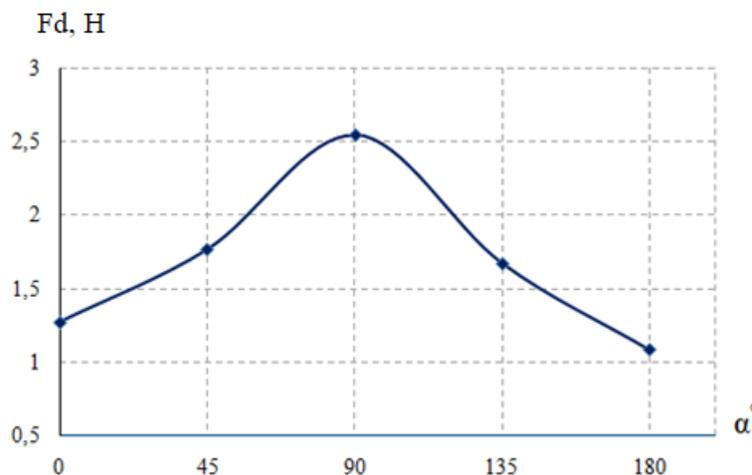
Figure 3. The results of measurements of the drag force from the angle of inclination at a flow rate of 5 m/s
