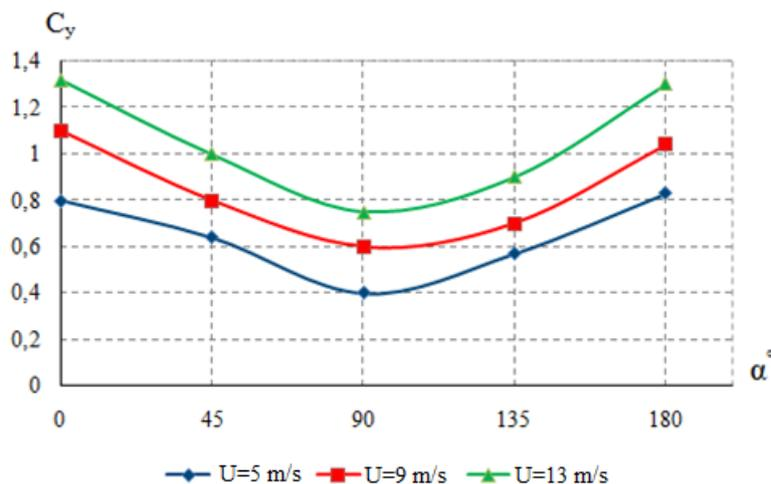
Figure 6. Change in the lift coefficient  $a$  depending on the angle of inclination at different flow rates
