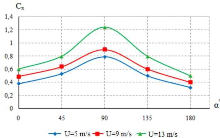
Figure 5. Change in the drag coefficient  $a$  depending on the angle of inclination at different flow rates
