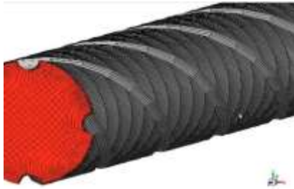
Figure 1. Calculation grid of the pipe with windings
