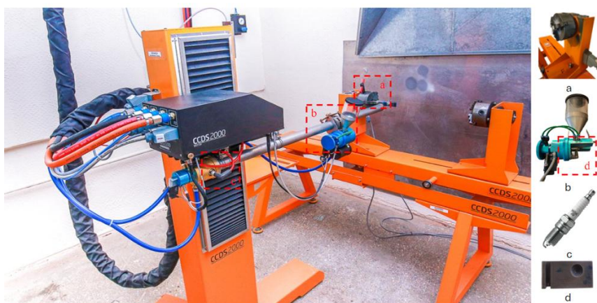
a — manipulator; b — powder dispenser; c — spark plug; d — dispensing plate
