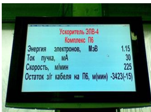
Figure 5. External status screen in the Podolsk cable plant
