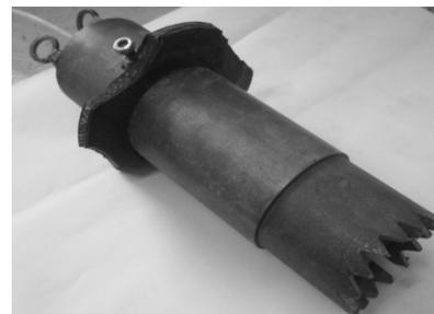
Figure 2. Appearance of electro-hydraulic drill
