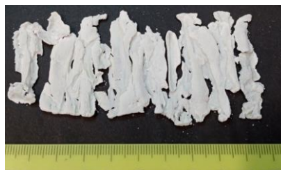
b) \text{Al}_2\text{O}_3 (816), \sigma_{\text{melt}}=0.26 \text{ g/cm}^2
