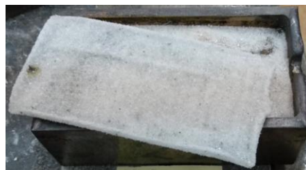
h) \text{SiO}_2 after treatment sand, \sigma_{\text{melt}}=0.59 \text{ g/cm}^2
