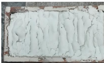
a) \text{Al}_2\text{O}_3 (816), appearance after irradiation, \sigma_2=0.94 \text{ g/cm}^2
