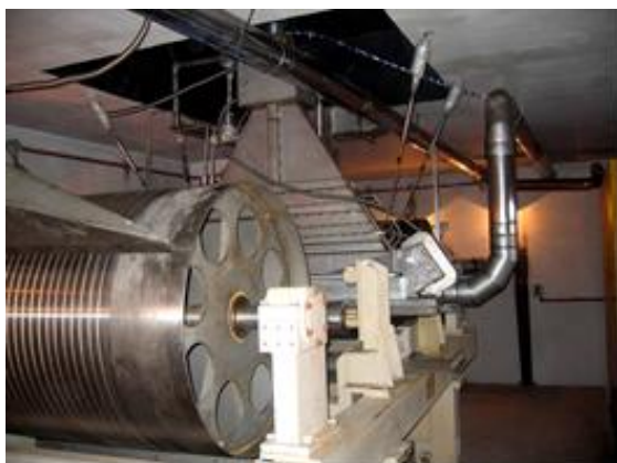
Figure 3. Extraction device with four-side irradiation system equipped
