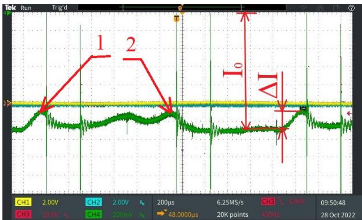
Figure 4. Oscillogram of the target current signal, with a beam current of I_0 = 15 mA and a beam energy of E = 2.5 MeV. The green beam is the total target current. The zero for the green signal on the oscillogram is located at the top; \Delta I = 2.3 mA is the value of the target current decrease. Peak 1 and 2 are the decrease in the total target current associated with the electron beam touching the opposite sides of the diaphragm holes.
