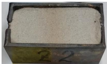
g) \text{SiO}_2 before treatment sand, \sigma_2=1.01 \text{ g/cm}^2
