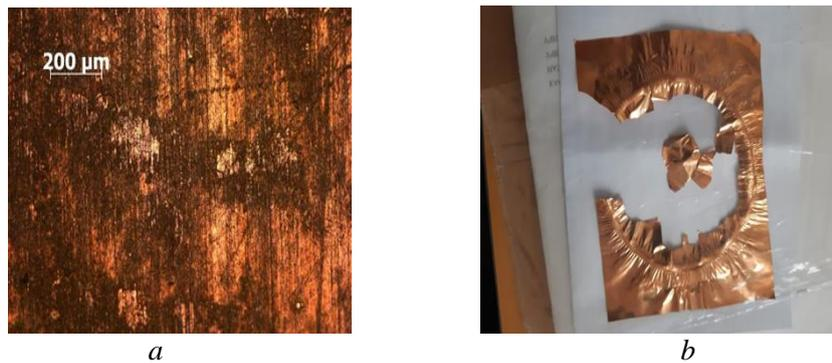
Figure 3. Fragments of a sample of copper foil before (a) and after (b) the magnetic field destruction test. The micrograph (a) shows traces of rolling, which confirms the X-ray diffraction picture
